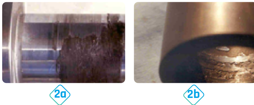
Figures 2a and 2b: Hard-chrome coated steel shaft, (a) and bearing with chrome residues (b)
