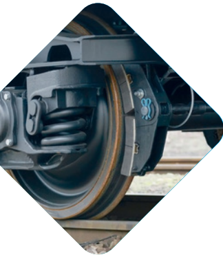
Backing plate = support of brake pad/lining
