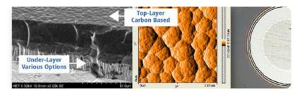
Topography of the top carbon layer depends on the morphology & and structure
