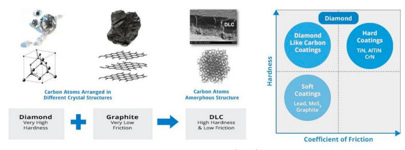
DLC coatings can be deposited using a diverse range of technologies and alloyed with elements such as hydrogen and metals such as chromium. These constituent elements and deposition technique can have a significant impact on the properties and structure of the DLC coating.
